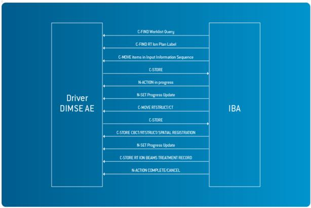
The scenario starts with a C-FIND query for Unified Procedure Steps from the treatment delivery device. The treatment delivery device can then take responsibility for the UPS by setting it to IN PROGRESS. Once the UPS is IN PROGRESS, the driver will only allows requests corresponding to the current session until the session has been completed by the treatment delivery device.
